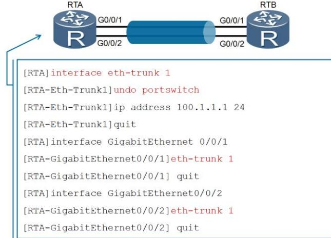
In order to configure layer 3 Link Aggregation on an Ethernet trunk link, it is necessary to transition the trunk from layer 2 to layer 3 using the *undo portswitch* command under the Eth-trunk logical interface. Once the *undo portswitch* command has been performed, an IP address can be assigned to the logical interface and the physical member interfaces that are to be associated with the Ethernet trunk link can be added.
