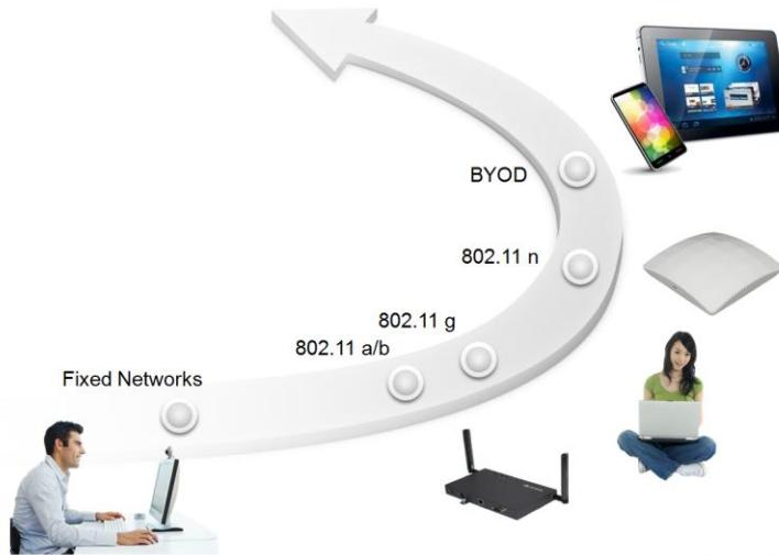
The evolution of enterprise networks involving WLAN have undergone three general phases since the 1980's, from fixed office, to supporting early mobile office solutions through the use of standalone access points (AP) that provided only limited coverage and mobility for users, to a more centralized form of WLAN involving management of multiple (thin) AP clients by a central controller.
