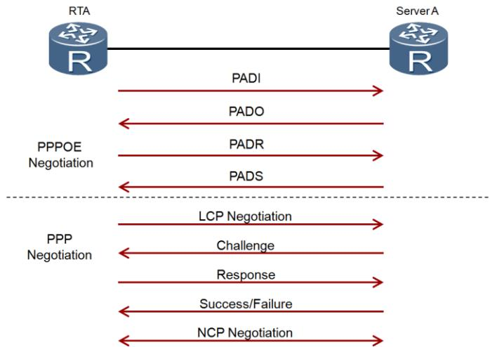
Once the PPPoE session begins, PPP data is sent as in any other PPP encapsulation. All Ethernet packets are unicast. The ETHER\_TYPE field is set to 0x8864. The PPPoE code must be set to 0x00. The SESSION\_ID must not change for that PPPoE session and must be the value assigned in the discovery stage. The PPPoE payload contains a PPP frame. The frame begins with the PPP Protocol-ID.
