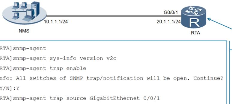
The SNMP agent is an agent process on a device on the network. The SNMP agent maintains managed network devices by responding to NMS requests and reporting management data to the NMS. To configure SNMP on a device, the SNMP agent must be enabled, for which the *snmp-agent* command is applied.
