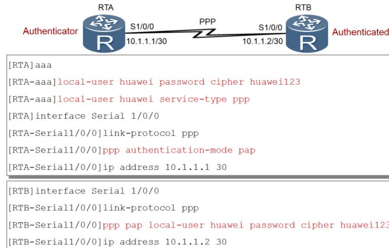
The establishment of PAP authentication requires that one peer operate as the authenticator in order to authenticate an authenticated peer. The PPP PAP authenticator is expected to define the authentication mode, a local user name and password, and the service type. If a domain is defined to which the local user belongs (as defined by AAA), the authentication domain is also expected to be specified under the PAP authentication mode.
