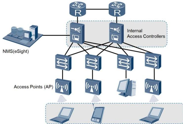
Wireless network deployment solutions over existing Ethernet networks commonly apply a two-layer architecture that is capable of meeting customer requirements, with minimal impact to the physical structure of the enterprise campus.
